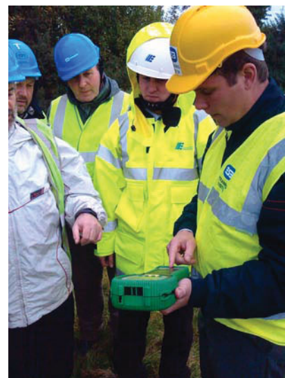
Measuring of earthing resistance.
