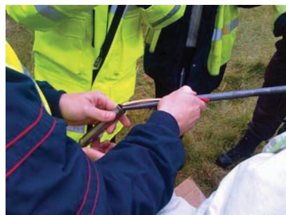
The earthing wire locks in the hardened steel tip with the leading rod.
